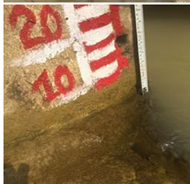
Figures 16, 17 & 18: Show how difficult it is to obtain accurate gauge readings
