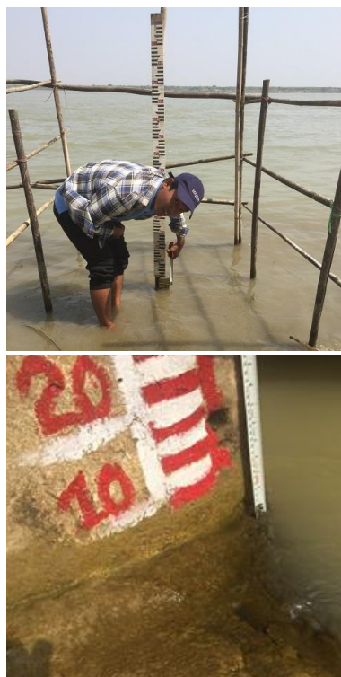
Figures 16, 17 & 18: Show how difficult it is to obtain accurate gauge readings
