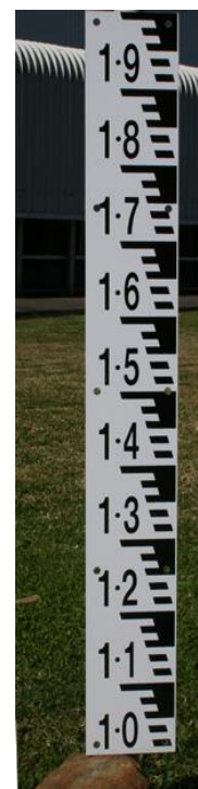
Figure 59: (Right) International standard gauge plates should be established wherever possible
