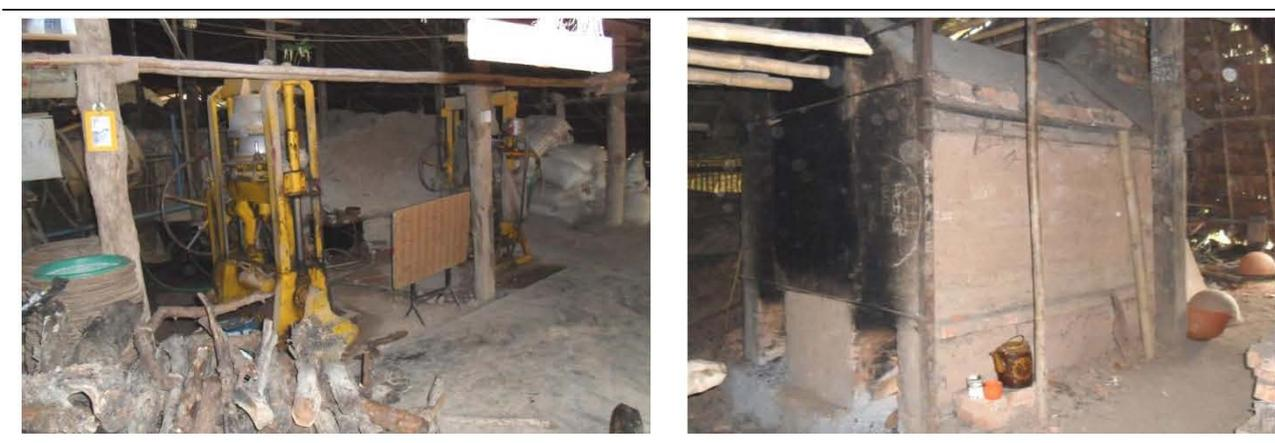
Hydraulic Clay moulding machine: for making water filters
