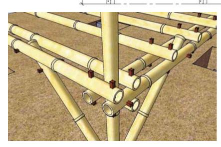
**Diagonal Bracings** Use 2" bamboo diagonal bracings at each corners
