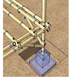
**Bamboo post Footing** Bamboo post shall be embedded at least 9" in the concrete foundation
