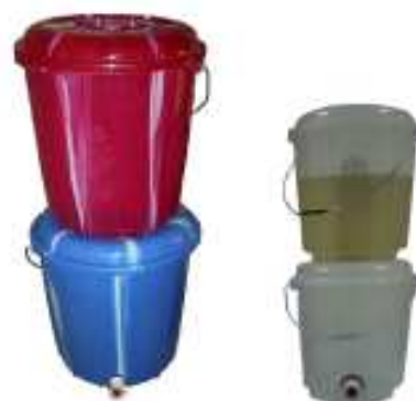
Two types of bucket filter: with two filter candles, as developed during the project (left) and with one filter candle, as already available in shops in Hajja (right)
