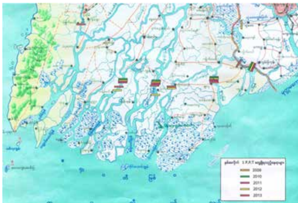
Figure 3.9 Map of the yearly maximum intrusion of the 1 ppt salinity concentration in the Ayeyarwady Delta for the period 2009 - 2013 (Hydrology Branch, Khon Ra, 2014).
