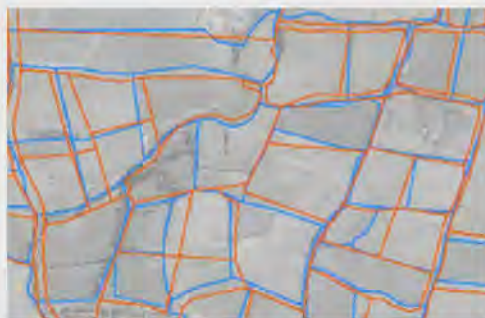
Digitized data plotted out to highlight difference in Kwin map and satellite image.
