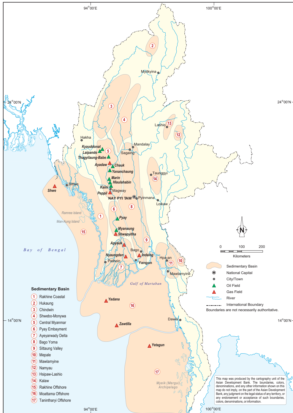
Figure A3 Location Map of Oil and Gas Fields in Sedimentary Basins of Myanmar
