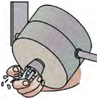
Push spring rod to release water from the pivoted container.
