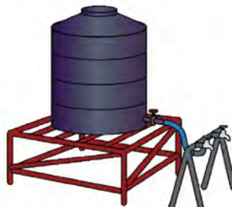
Water tank mounted on frame
