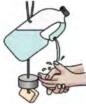
Tip the bottle and pour water into the handle. When the bottle is released water will slowly empty from a hole in the handle. The can is used to protect the soap from the rain.
