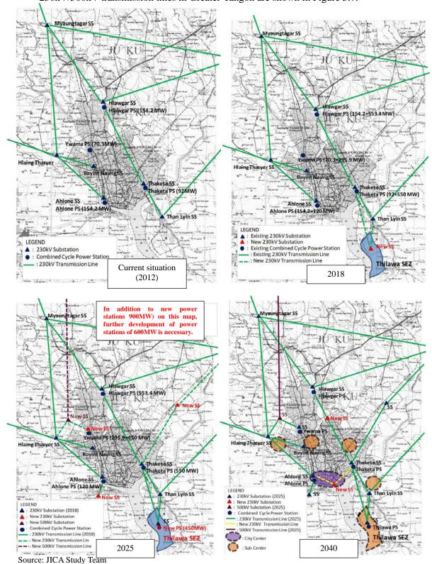
Figure 5.7: Plan of 230kV/500kV Transmission Line and Power Station in Greater Yangon
