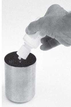
Add 20 drops (approximately 1ml) of methanol
