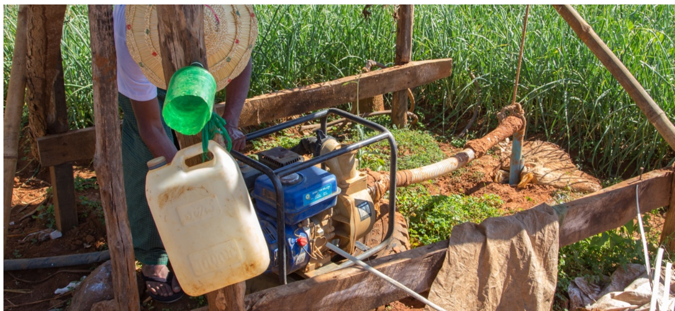
Figure 20: Pinlaung township, Inn Gaung village. Low cost shallow (30ft) tubewell with 2" diameter petrol pump irrigates about half an acre.
