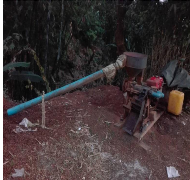
Figure 8 and 9: Coffee milling in Thandaunggyi area using traditional hand pound for polishing and small rice milling machines for milling
