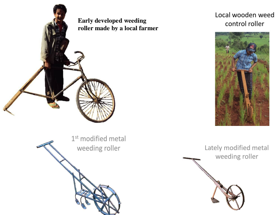
Figure 4. Weeding rollers models developed in partnership with FFS participants
